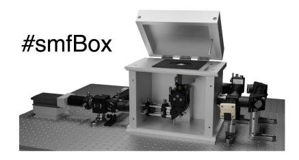
'3D model of the completed smfBox, with the front panel of the microscope body removed' taken from Ambrose, B. et al. (2020) https://doi.org/10.1038/s41467-020-19468-4 [1]
