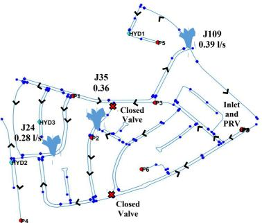
Figure 2. The True system state illustrating the leakage hotspot locations and flows, the closed valves, sensor locations the flushed
