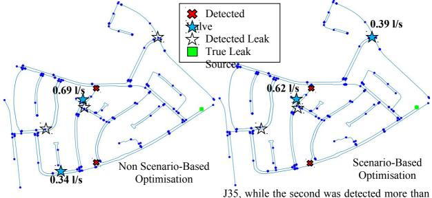
300 m away from the closest leak J24. This led to an incorrect detection of emitter values. The best solution was reached after 1081 seconds. On the other hand, when a scenario-based method was used a fitter solution of F=0.82 was achieved only after 224 seconds. The J109 was correctly detected in terms of location and emitter flow, while the
